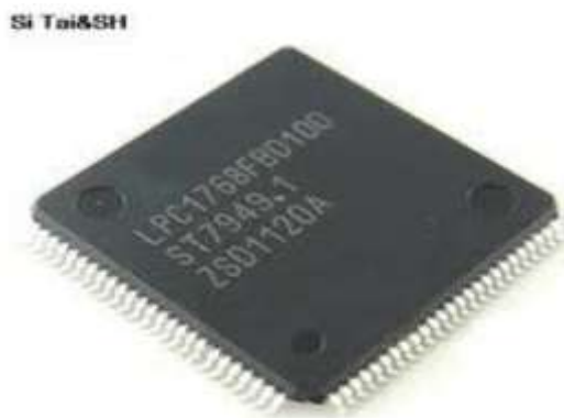
Fig 6.1 LPC1769 ARM cortex M3 micro- controller
